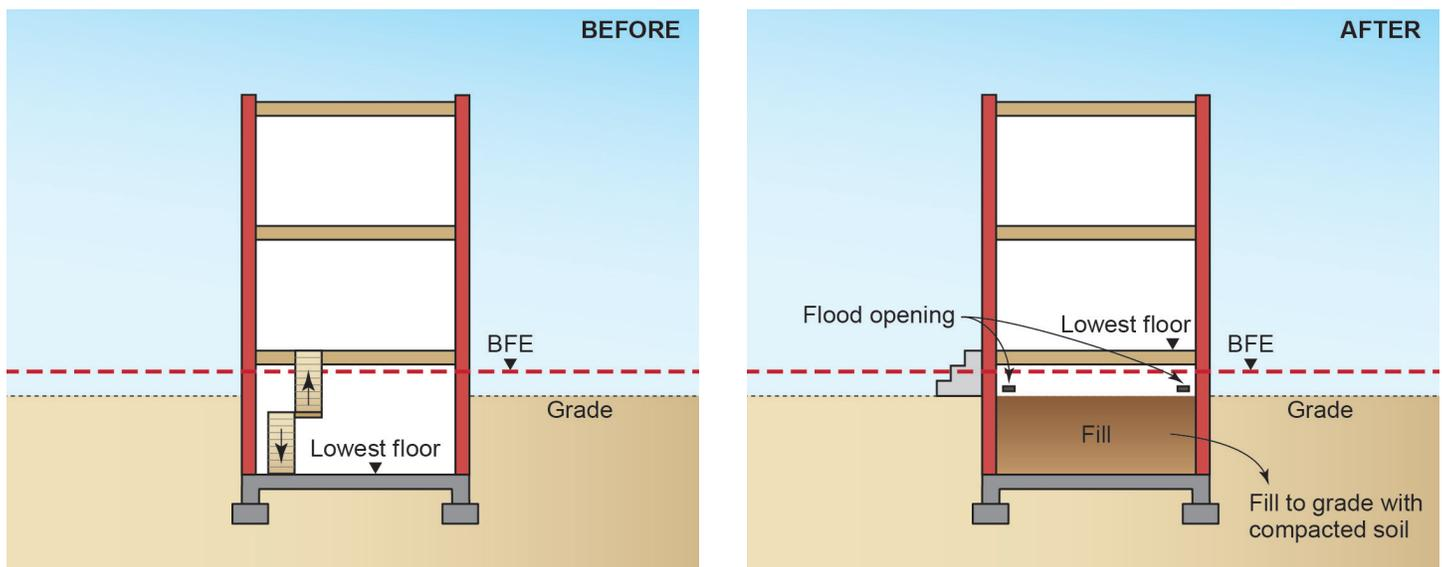
Figure 1: Basement infill before and after mitigation
