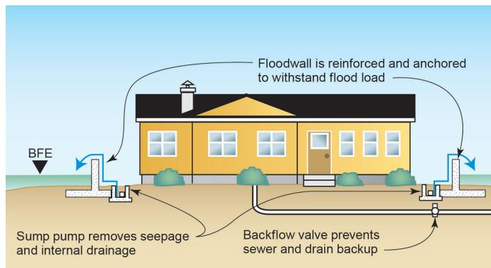
Figure 9: Residential floodwall
