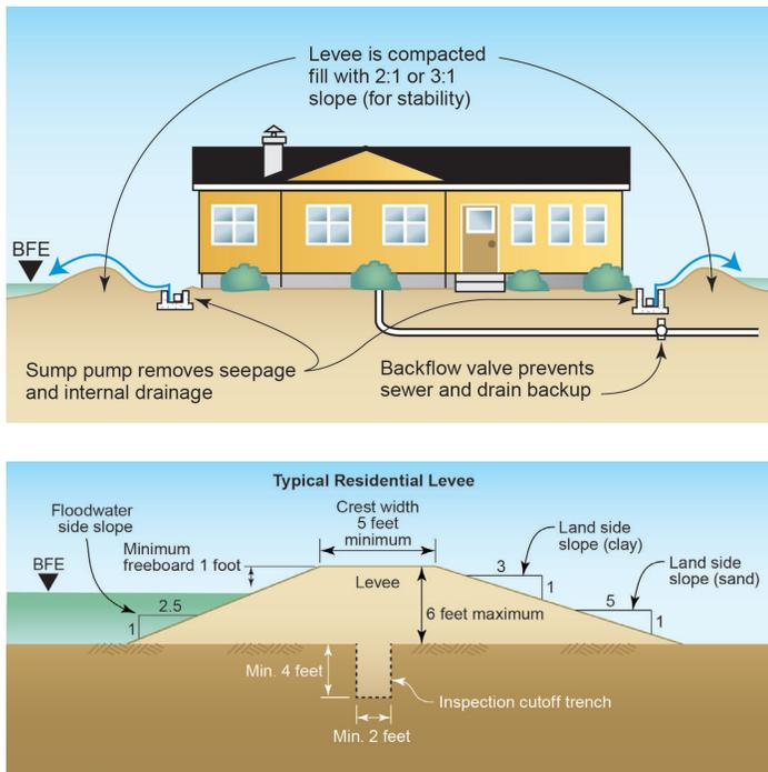
Figure 10: Residential levee and typical levee cross section
