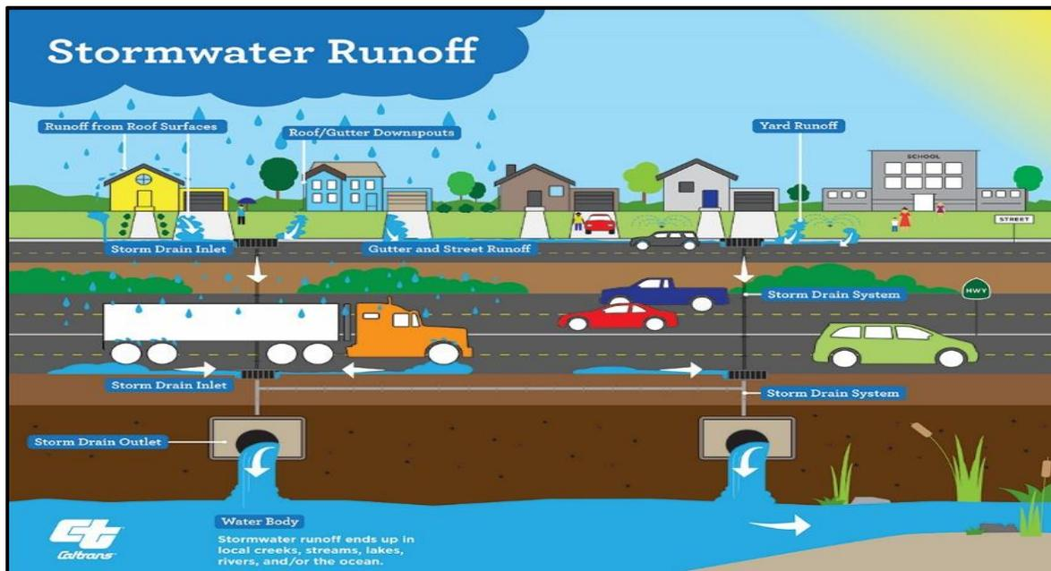
*The storm drain system, as shown above, is made up of curb inlets, pipes and open ditches. This system is designed to funnel untreated rain water to local waterways.*
